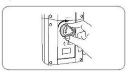
Reset the emergency stop by turning the button in the direction indicated by the arrows.
