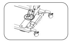
10. Pull up the folding hand shank to fold the lift mast down.
