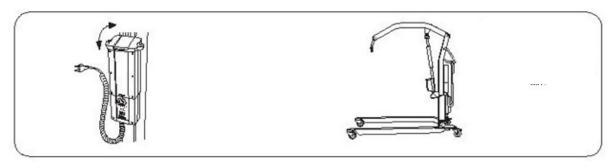
7. Mount the holder for the charging cable. Hook it on the outer edge and press down until you hear a 'click'.
