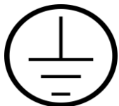
Protective Earth Ground Symbol
