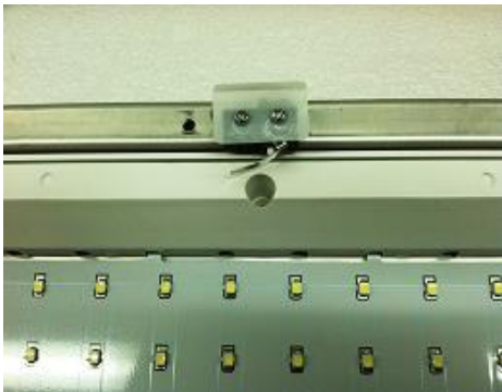
Micro Switch, built-in at the metal frame
