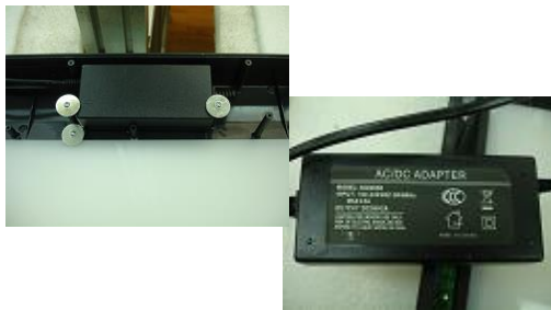
External Power Adaptor at inside Poor Construction to built-in
